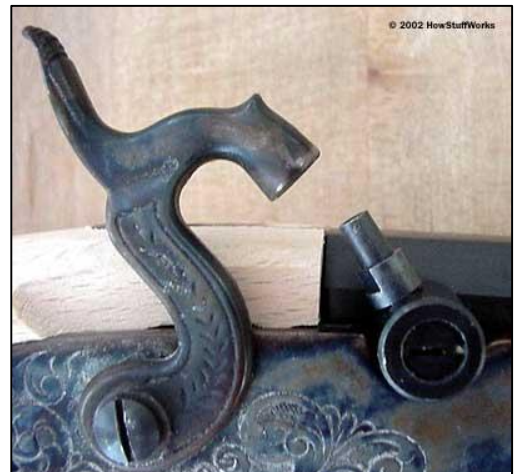
The percussion hammer in a cocked position. The cap, about the size of a pencil eraser, fits over the end of the nipple. www.science.howthingswork.com
